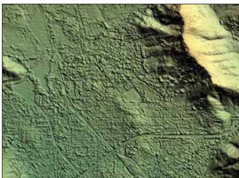
Digital Surface Model Resolution: 5m Vertical Accuracy: 1m LE90%
