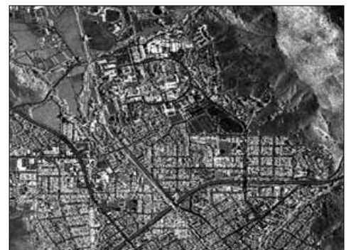
Orthorectified Radar Image Resolution: 1.25m Horizontal Accuracy: 4m CE90%
