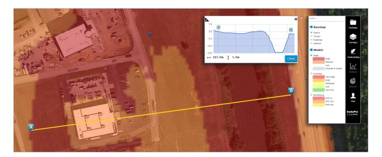
InsitePro's interactive elevation tool enables terrain profiling capabilities that help users understand the shape of the ground at a location, providing insight into where water will flow around a property. This also allows them to compare elevations of river banks to discern where rivers will overflow first. The distance measuring tool allows them to measure distances and elevation differences between properties and hazards.
