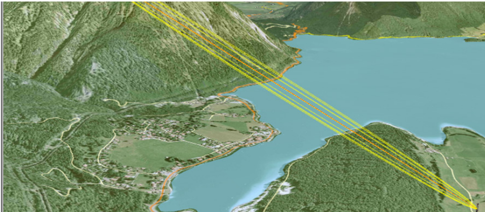
Example of point-to-point microwave link fresnel zone profile using NEXTMap 3D terrain data
