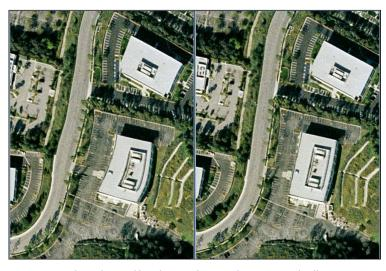
Intermap's Orthorectification engine used to geometrically correct sensor distortions in airborne and satellite derived imagery. Comparison in Orange County, CA, using the USGS NED data (left) and Intermap's high-accuracy DEM (right)
