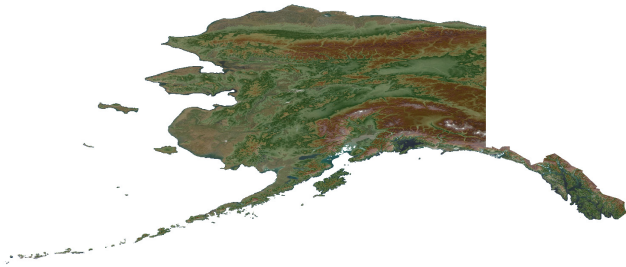
Intermap collected the majority of the elevation data for the Alaska program. All data meet USGS 3DEP specifications with 5-meter resolution and high-accuracy elevations for the entire state.
