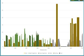
NEXTMap Clutter provides full clutter height and classification. The terrain in this profile is colorized based on classification. The brown buildings are easily discernable from the green vegetation.
