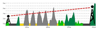
NEXTMap Clutter provides full clutter height and classification. The terrain in this RF profile is colorized based on classification. The grey houses are easily discernable from the green vegetation.
